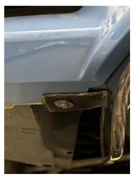
6. After securing the middle section of the diffuser, use the provided double sided tape to help align the side pieces of the diffuser kit to the contour of the car's body lines and the diffuser.
