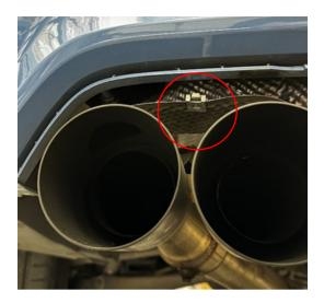
5. Reinstall the middle part of the diffuser and use the provided hex screws to secure it to match the location of the clips. As well as using the stock hardware to secure the sides of the middle diffuser piece.
