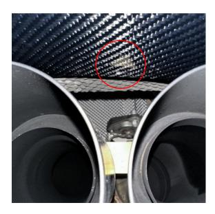
4. After removing the diffuser, slide the provided clips on the heat shield and line them up with the locations determined in the previous step.
